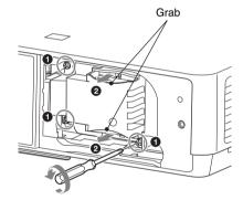
4 Insert the new lamp all the way in until it is securely in place (1). Tighten the 3 screws (**2**).
